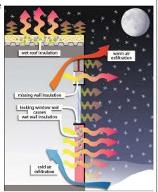
used to make the building perform better. The primary purpose of an air barrier system is to stop the air from leaking into and out of the building enclosure.
