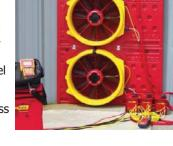
Test programs conforming to USACE protocols and requirements for measuring air leakage in buildings, including ECB 2009-29 Building Air Tightness Requirements.
